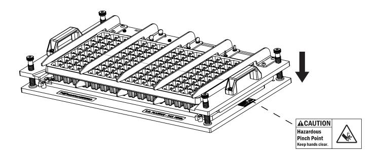
8. Using both handles, press top plate down to allow base board pins to penetrate drainage holes of plug tray to dislodge plugs from bottom of tray.
