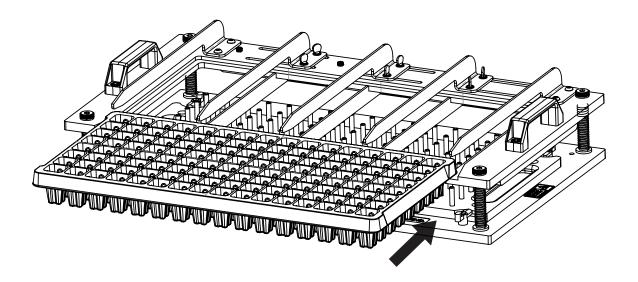
7. Slide plug tray into top plate between upper and lower support ribs from frame front.
