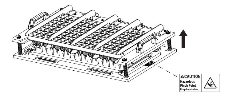
9. Release pressure on handles to return top plate to resting position.
