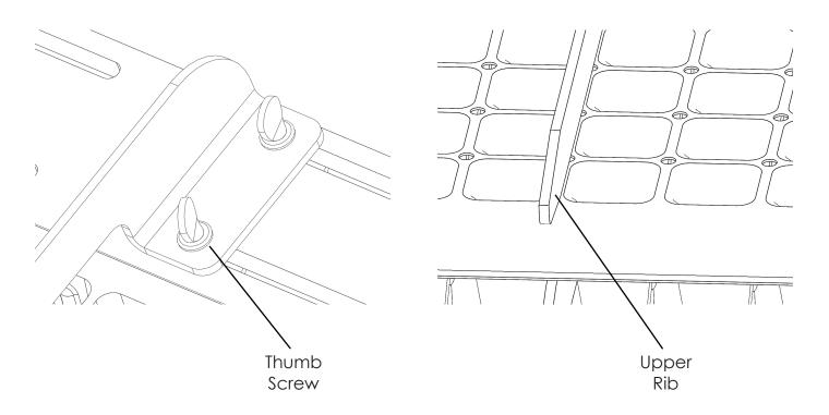
6. To adjust upper support ribs, loosen thumb screws and slide to align between cells of plug tray. Tighten to hold in place.
