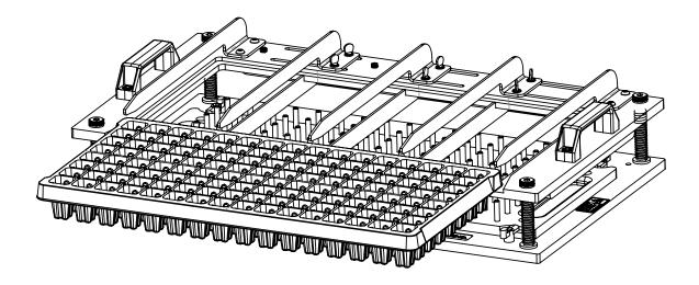
4. Align lower and upper support ribs between cells of plug tray.
