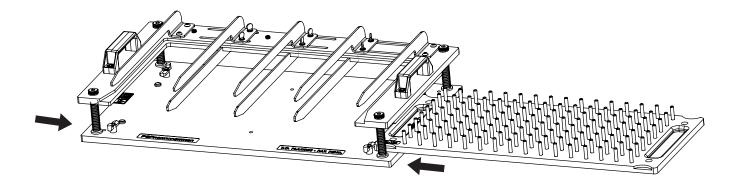
1. Slide base board into bottom plate of frame from either side (right or left).
