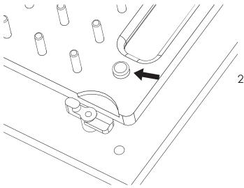
2. Align (4) holes in base board with (4) dowel pins in bottom plate.
