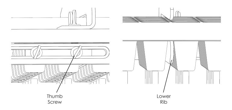
5. To adjust lower support ribs, loosen thumb screws and slide to align between cells of plug tray. Tighten to hold in place.
